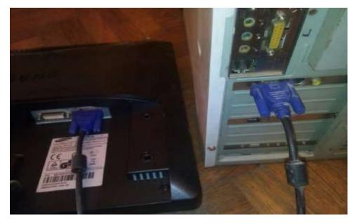
Step 2: Connect the spare VGA cable.
